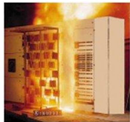
Internal arc test
