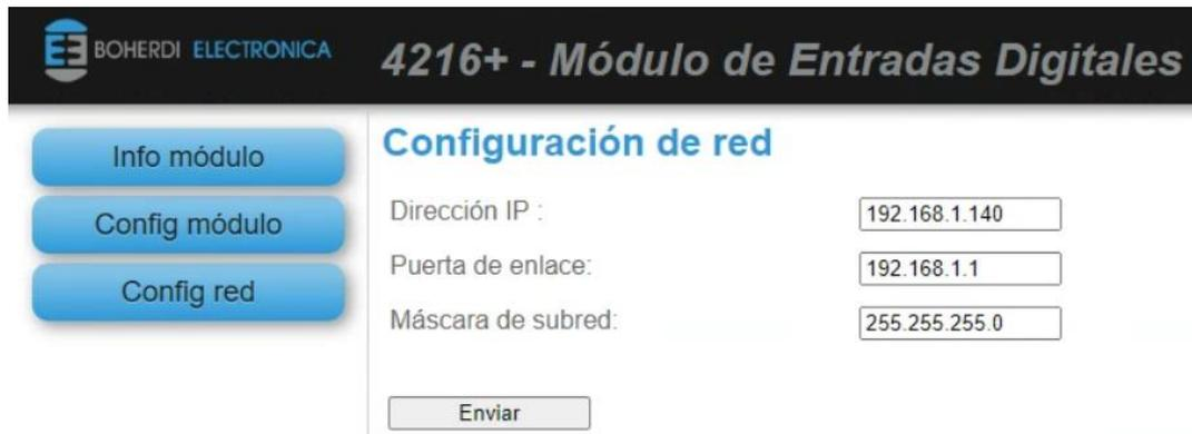
The screenshot shows the 'Configuración de red' (Network Configuration) page. On the left, there are three blue buttons: 'Info módulo', 'Config módulo', and 'Config red'. The main area is titled 'Configuración de red' and contains three input fields for network parameters:
